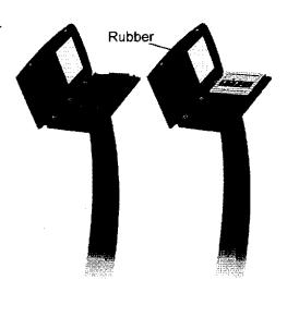
4: Connect power cable onto iPad, close the front cover and lock it.
